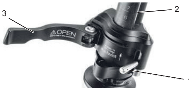
Figure 58: Opened clamping lever on the stem quick release (3) on the stem (2), version I, with locking lever on the stem (1)
