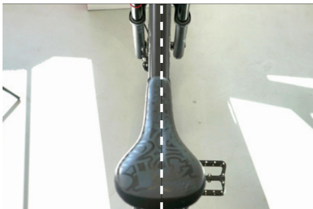
Figure 80: Positioning the saddle in direction of travel
