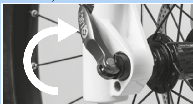
Figure 75: Closing the quick release
