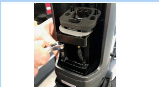
Figure 48: Removing the 4 mm hexagon screws
