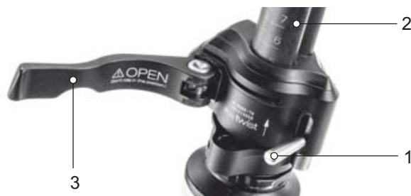
Figure 135: Opened clamping lever on the stem quick release (3) on the stem (2), version I, with locking lever on the stem (1)
