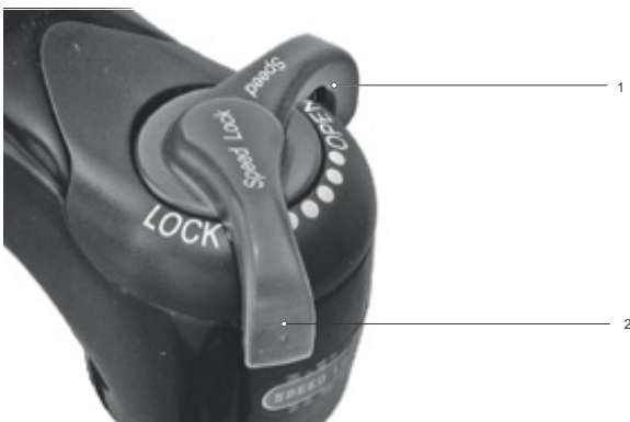
Figure 228: Changing compression adjuster to a harder setting
