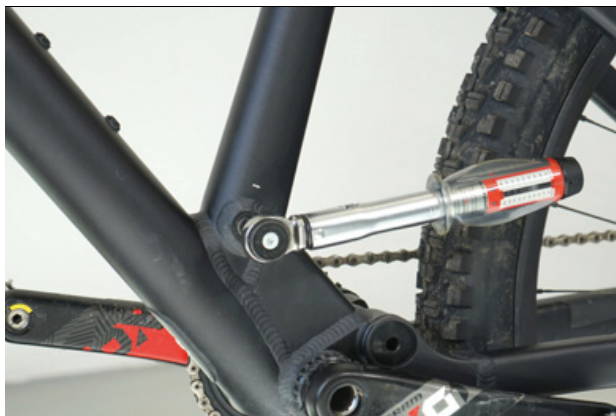
Figure 81: Tightening the seat post axle
