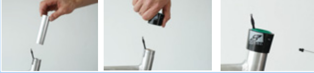
Figure 212: Fitting the slide bushing and outer sleeve
