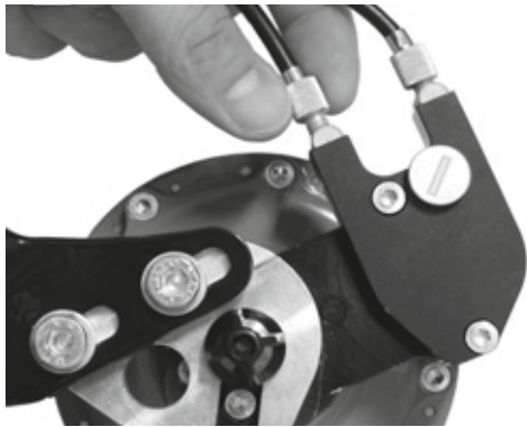
Figure 148: The tension adjuster on Rohloff hub versions with external switch control is located on the cable box positioned on the left-hand side
