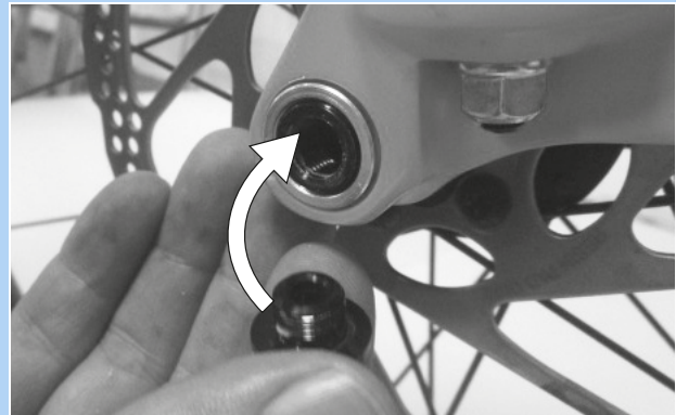
Figure 52: Pushing the quick release lever into the axle
