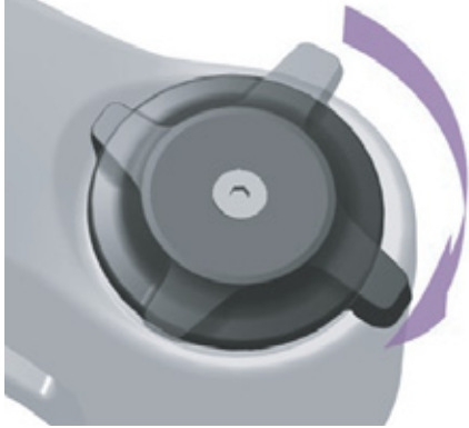
Figure 132: Changing compression adjuster to a harder setting
