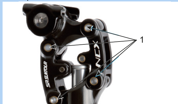
Figure 154: SR Suntour suspension seat post lubrication points
