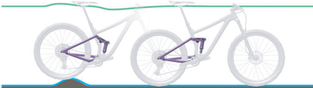
Figure 105: Optimum rear frame damper ride performance over bumps
