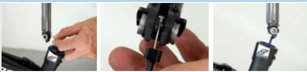
Figure 213: Attaching and pushing in the seat post
