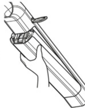
Figure 121: Battery is unlocked
