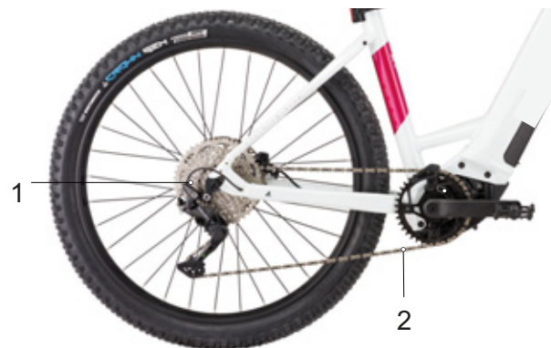
Figure 32: Chain drive with derailleur gears
