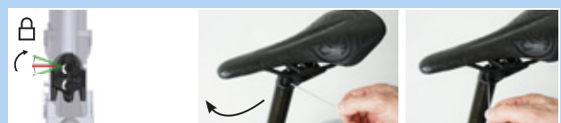
Figure 192: Closing the height adjustment
