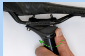
Figure 211: Closing the height adjustment
