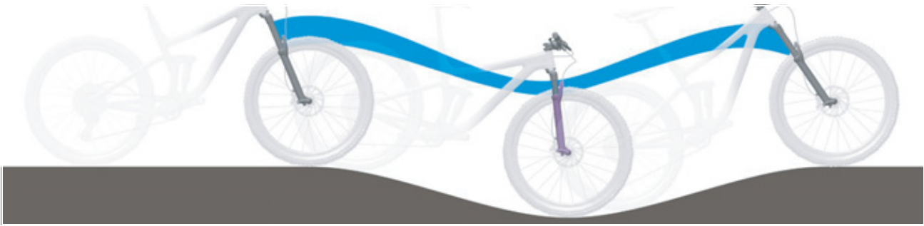
Figure 221: Excessively soft suspension in the suspension fork on hilly terrain
