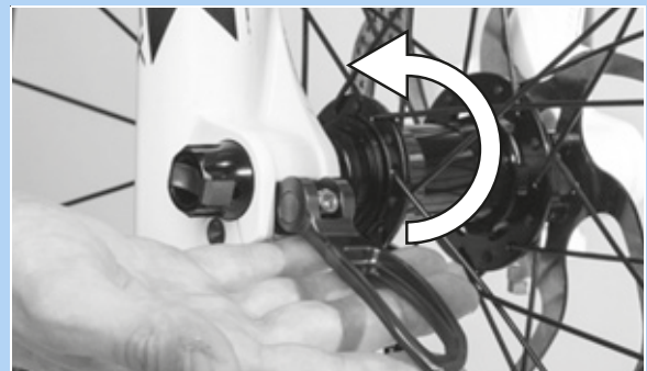
Figure 57: Pressing the quick release lever in the direction of the arrow
