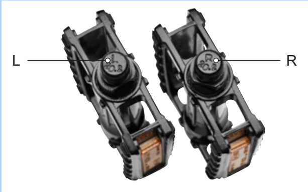
Figure 64: Example of markings on pedals
