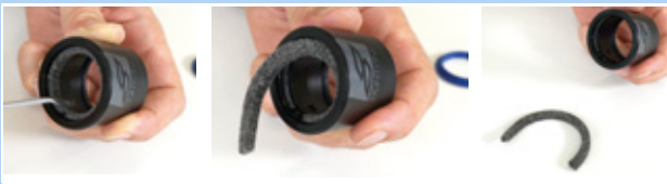
Figure 201: Removing the felt ring
