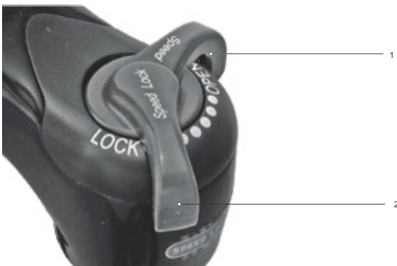
Figure 222: Changing compression adjuster to a harder setting
