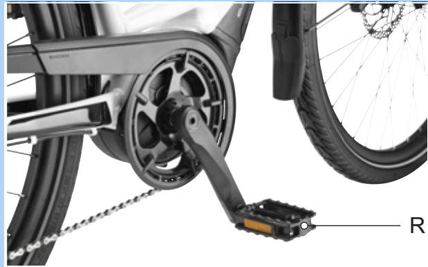
Figure 66: R-pedal in the right-hand crank arm
