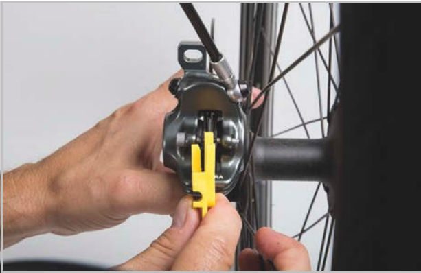
Figure 140: Checking the brake lining when fitted with the help of the transport safety wear gauge
