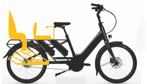
Figure 107: A child seat at the rear and a saddle seat with sideblades in front, suitable for one young child (1–6 years old, 9–22 kg) and an older child (6–10 years old, 18–38 kg)
