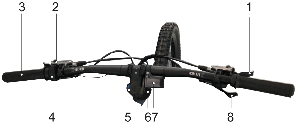
Figure 42: Detailed view of handlebars with SHIMANO SC-E800 on-board computer, used as example
