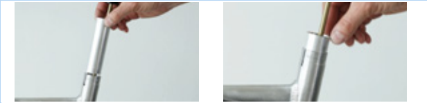
Figure 197: Inserting the slide bushing tube into the seat tube
