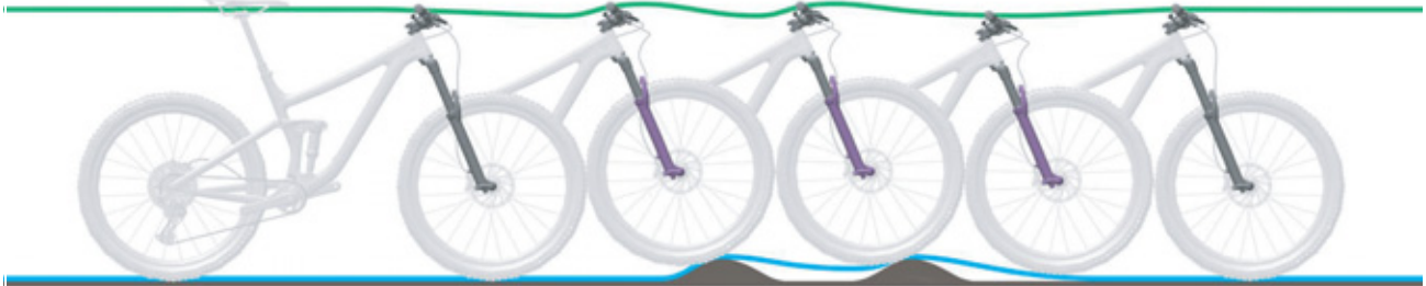
Figure 230: Suspension fork rebounding too slowly
