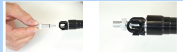
Figure 183: Screwing the valve adapter in
