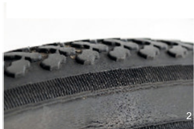
Figure 154: Examples of fatigue cracks (1) and ageing cracks (2)
