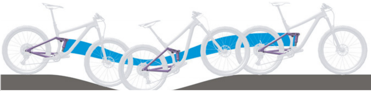
Figure 240: Excessively soft suspension in the rear frame damper on hilly terrain
