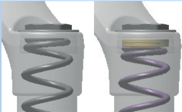
Figure 89: Screwing and unscrewing the preload adjustment ring
