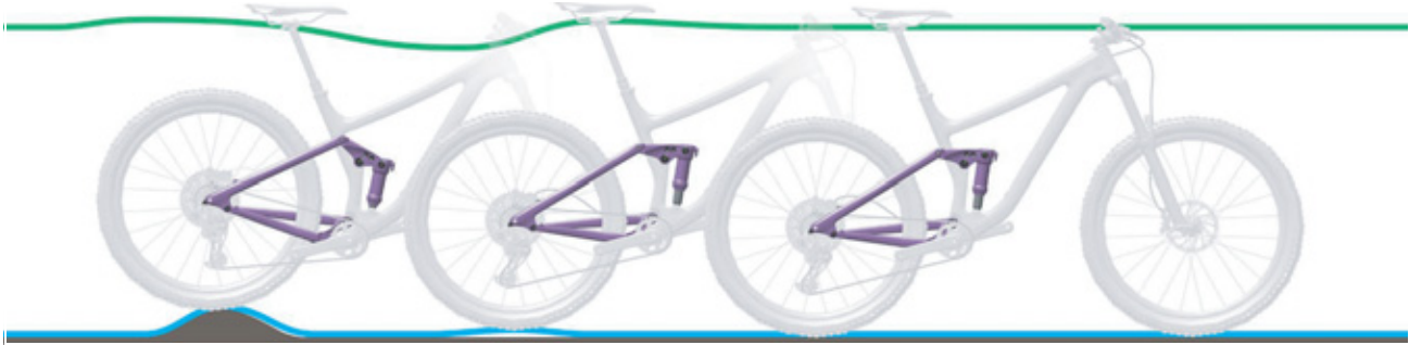
Figure 236: Rear frame damper rebounding too quickly
