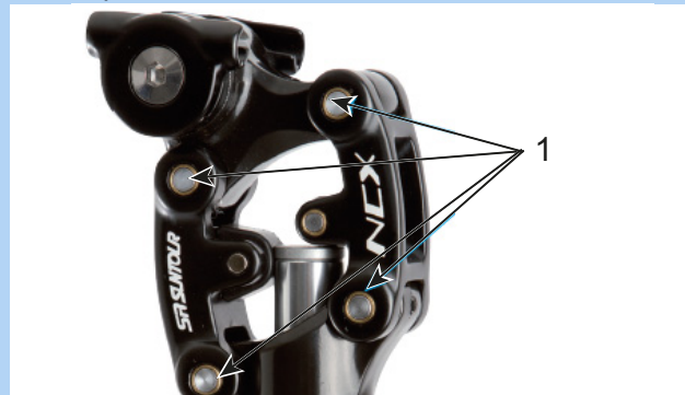
Figure 165: SR Suntour suspension seat post lubrication points
