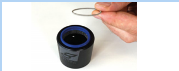
Figure 210: Removed spring washer
