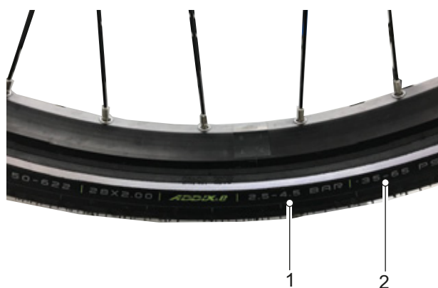
Figure 152: Tyre pressure in bar (1) and psi (2)
