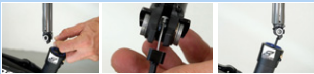
Figure 224: Attaching and pushing in the seat post
