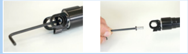
Figure 182: Unscrewing the valve cap
