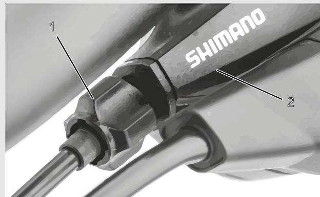
Figure 67: Adjusting sleeve (1) for the single-cable, cable-operated gear shift with shifter housing (2), example
