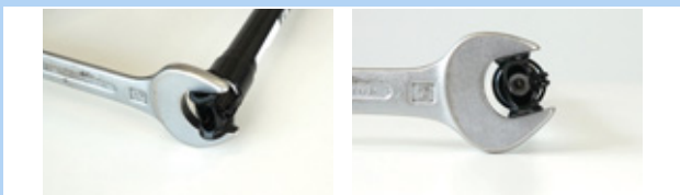
Figur 182: Sikring mod at dreje
