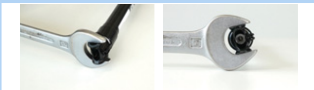
Figur 198: Sikring mod at dreje
