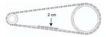
Checking the chain and belt tension
