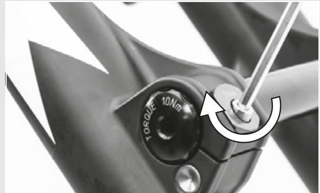
Figure 27: Tightening the securing clip
