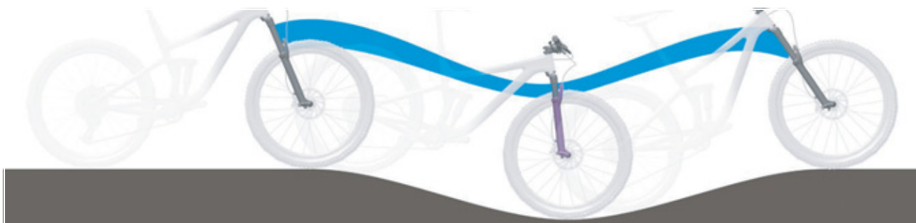
Figure 93: Excessively soft suspension in the suspension fork on hilly terrain
