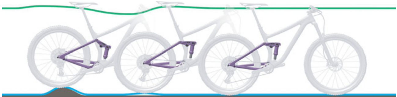
Figure 97: Rear frame damper rebounding too quickly
