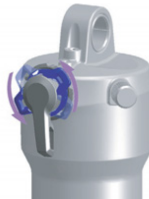
Figure 72: Changing compression adjuster to a softer setting
