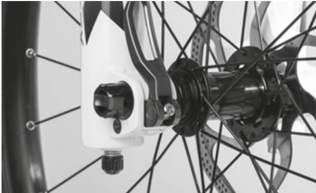
Figure 84: Adjusting the quick release clamping force
