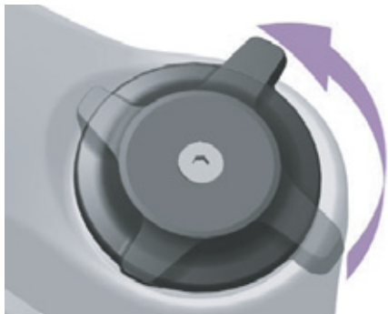
Figure 79: Changing compression adjuster to a softer setting
