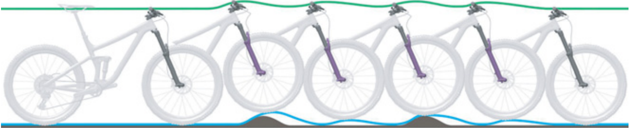
Figure 89: Suspension fork rebounding too quickly
