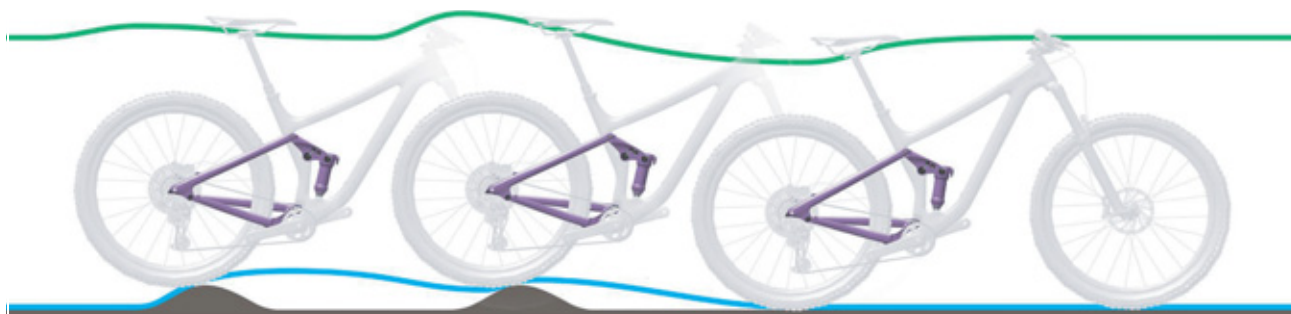
Figure 99: Rear frame damper rebounding too slowly
