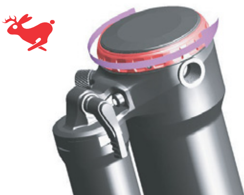
Figure 100: Turning rebound damper towards hare symbol
