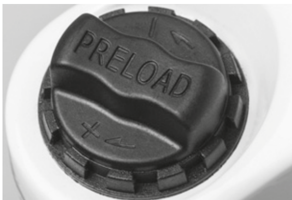
Figure 53: Sag setting wheel on the suspension fork crown
