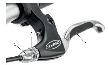
Brake lever (1), lock nut (2) and setting bolt (3) of the cableoperated rim brake
