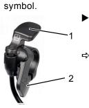
To release the front wheel suspension, push the side unlocking lever.
