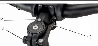
Stem, version II with clamping lever (1), unlocking knob (2) and knurled nut (3)
