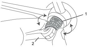
Wheel quick release, version IV, with twist knob (1) and clamping lever (2)
