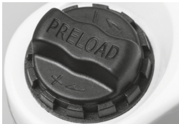
Figure 57: Negative deflection setting wheel on the suspension fork crown
